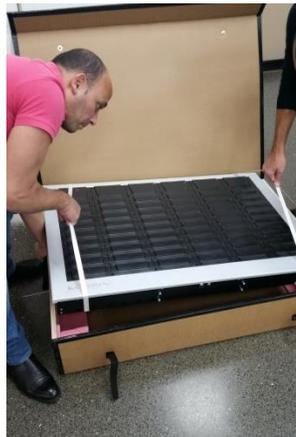
5) Lift the unit from both sides and hang it with the hooks until it is hanged secured
