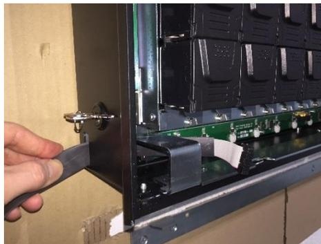
5. Connect the flat cable connector to the connector in the Pod board. Make sure it is firmly connected
