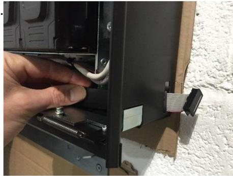
4. Drive the flat connector cable into the Pod through the designated hole.
